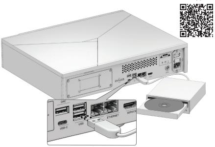
Note: An M.2 NVMe SSD must be installed to enable CD ripping.
